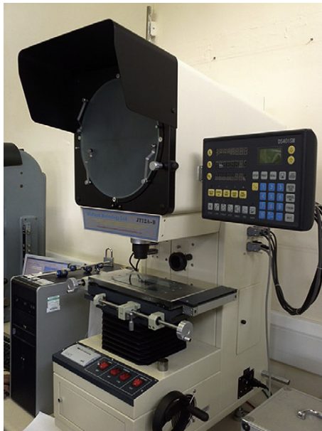
Figure 9.15 Typical profile projector with digital display. (Courtesy Staffordshire University)
